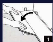
LIFT Insert Plank into Channel
